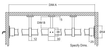
/CPD - Double coupler. See page 3 for details. Specify Dim A, B and C
