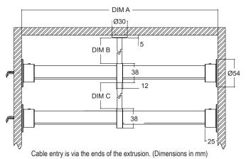
/CP - Coupler is required when the hanging rail exceeds 3m. In this case 2 lengths will be supplied and the coupler hides the join allowing up to a 6m hanging rail. Cable entry will be required at both ends. See page 3 for details. Specify Dim A and B
