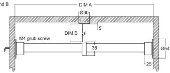
/CSD - Double centre support is required for two lengths over 1.2m. Specify Dim A, B and C
