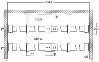
Cable entry is via the ends of the extrusion. (Dimensions in mm)
